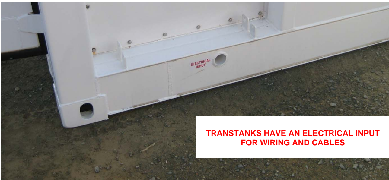
A view of the Pump Bay showing Electrical Input
